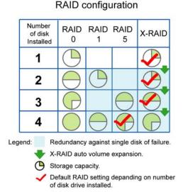
X-RAID is Infrant Technologies patent-pending Expandable RAID technology, allows users to add drives at their leisure. Start with one disk or add a second disk to gain disk failure protection. Add a third to automatically double the capacity while maintaining protection. Finally, add a fourth disk to triple the protected capacity, all without reconfiguring the system and without having to shuffle data in and out of the device.
