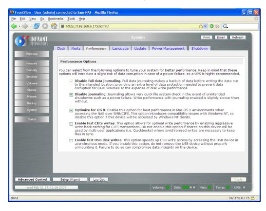
**Disable Full Data Journaling** – As mentioned above, with this option, you run the risk of the RAID Write Hole, where a portion of the data is written, but the rest is not, and the parity bit is incorrectly calculated.
